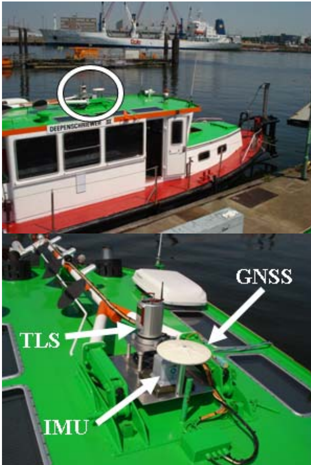
Fig. 10: Installation of TLS Riegl VZ-400 onboard the “Deepenschriewer III”.
