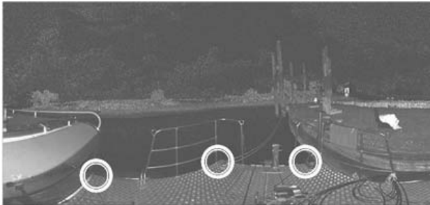
Figure 6: Spatial resection for the determination of the scanner position in the coordinate system of the "Level-A" using control points (bright circles). The image is presented as intensity values.
